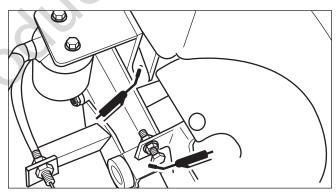
Figure 21. Suspension & Deck Lift Pivots
